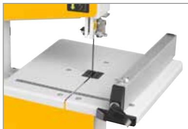
Maximum cutting capacity up to 80 mm
